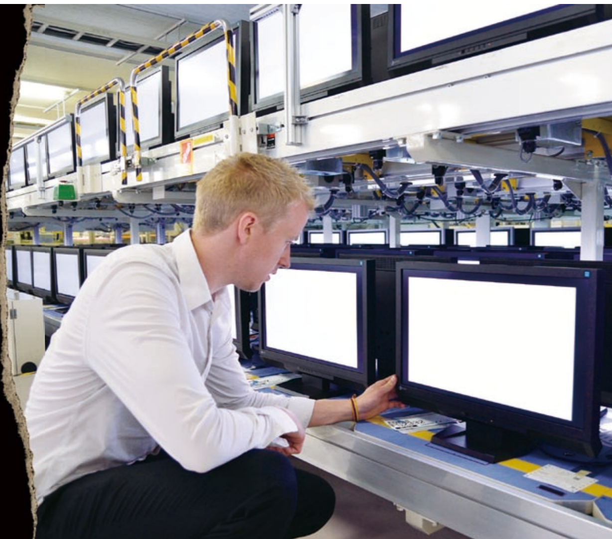
Checking out monitors undergoing the aging process, which insures that the display and electronics are stable before they are adjusted.
